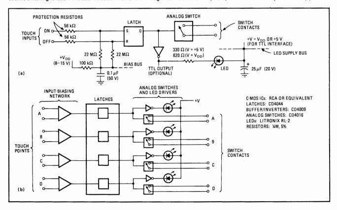
cuit's TTL interface must be sacrificed. two contacts will assure triggering. Also, to eliminate any chance of damage to the flip-flop inputs from an ex-In remote locations, where power lines or other major electromagnetic-field sources are not available, it is adternal power source, the inputs should be protected visable to install a second contact (at ground potential) against excessive current flow with 56-kilohm resistors, on each sensor, so that a slight conduction between the as shown.
